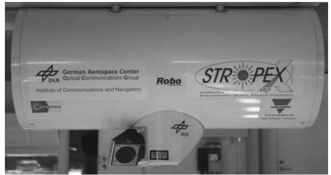
Fig. 8. Free-Space Experimental Laser Terminal (FELT) [3].
