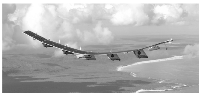
Fig. 4. Unmanned solar powered plane Helios [18].
