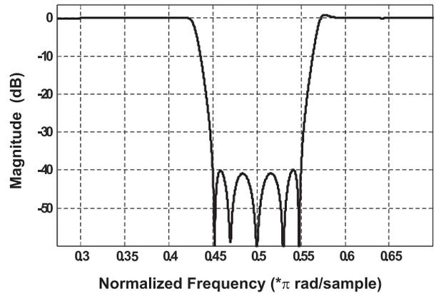
Fig. 7. Magnitude frequency response of the bandstop filter.
