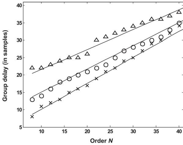
Fig. 3. The values of  $\tau_1$  versus  $N$  for lowpass filters with  $M = 4$  and  $\omega_t = 0.04\pi$  obtained for:  $\omega_{pw} = 0.05\pi$  ( $\Delta$ ),  $\omega_{pw} = 0.1\pi$  (o),  $\omega_{pw} = 0.2\pi$  (x), and its approximation (solid lines) by (5).
