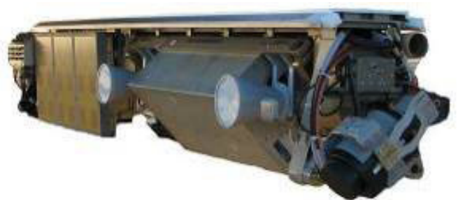
Fig. 5. X + L bands and visible-band camera configuration.
