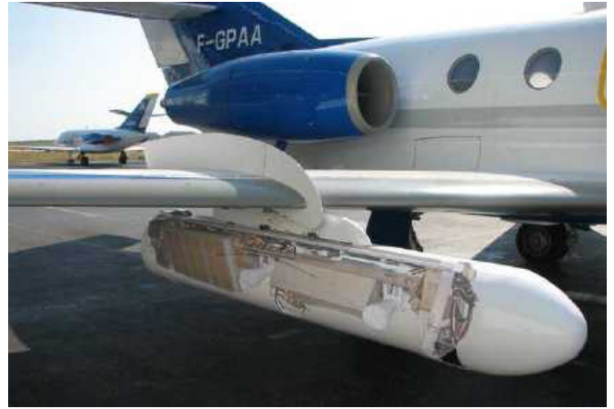
Fig. 4. Cutaway view of a SETHI pod.
