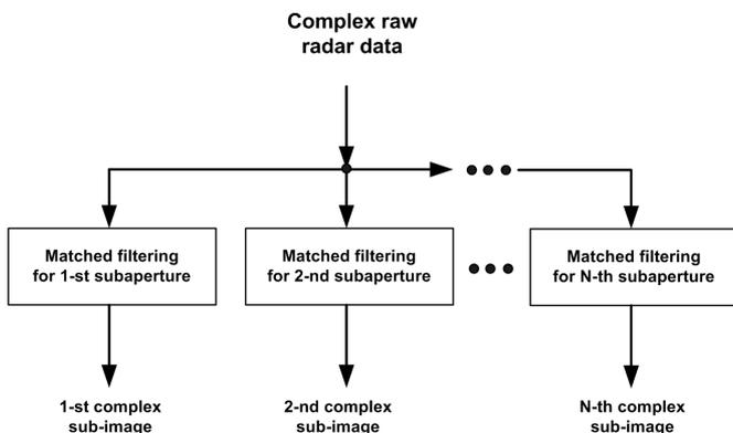
Fig. 3. Simplified block diagram of the multilook processing.
