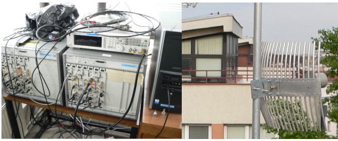
Fig. 6. Measuring Equipment – Agilent and High Gain 2.4 GHz antenna on the right.
