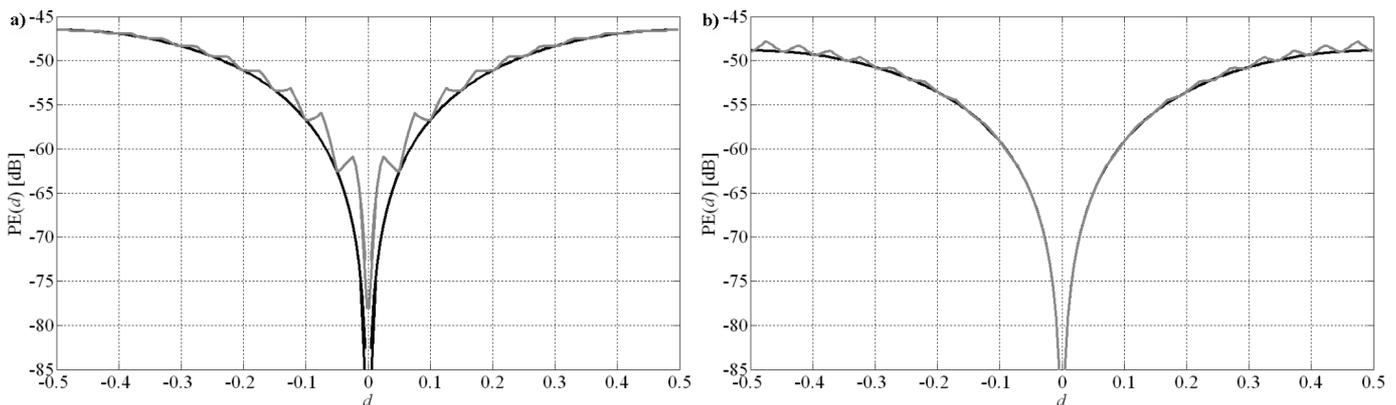
Fig. 11. PE for minimax variable fractional delay filters with  $f_a = 0.42$  (black lines) and their equivalents designed using set of 10 asymmetric reference windows stored in a look-up-table (gray lines). Filters lengths  $N = 18$  (a) and  $N = 19$  (b).
