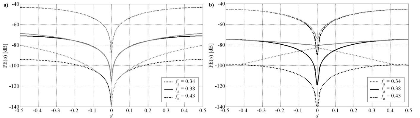
Fig. 9. PE for minimax variable fractional delay filters (black lines) with  $N = 19$  (a) as well as  $N = 20$  and their equivalents with discarded odd part of extracted windows (gray lines). Filter gain correction is not applied.
