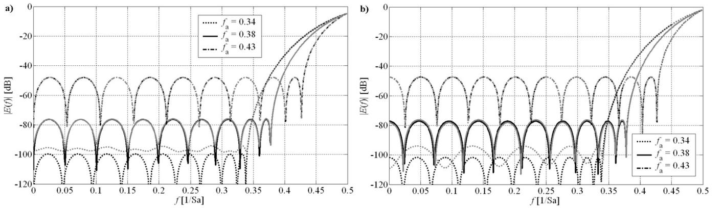
Fig. 8. Magnitudes of complex approximation errors for minimax fractional delay filters (black lines) with  $N = 19$ ,  $\epsilon = -0.2$  (a) as well as with  $N = 20$ ,  $\epsilon = -0.2$  (b) and their equivalents with discarded odd part of extracted windows (gray lines). Filter gain correction is not applied.
