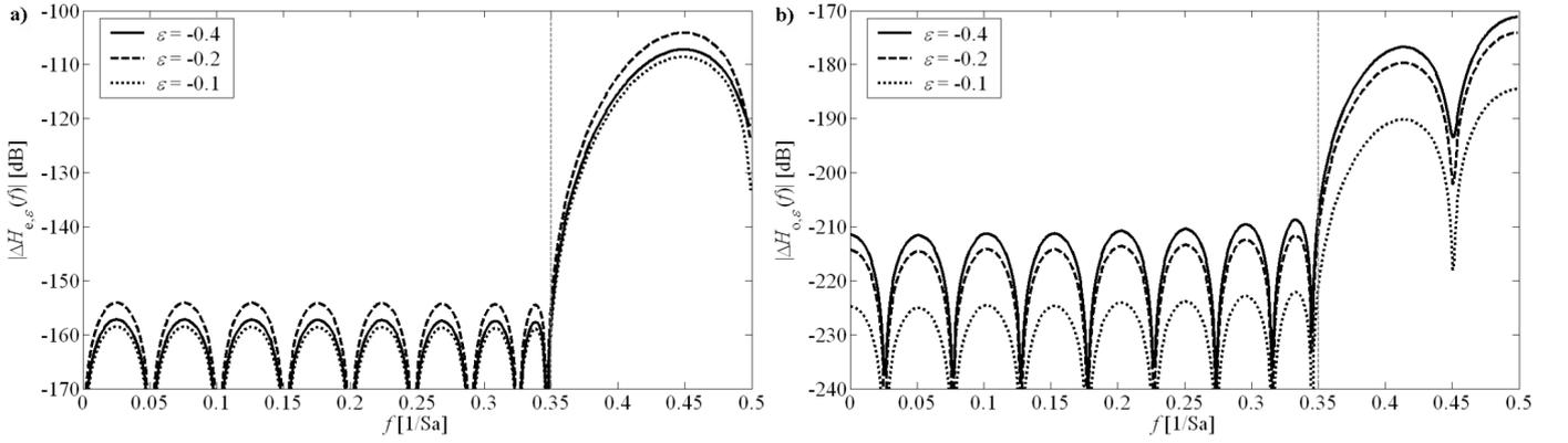
Fig. 7. Magnitude responses of reconstruction errors of optimal filter related to even (a) and odd (b) parts of reference window for different net delays. Reference window extracted from filter with  $N = 19$  and  $f_a = 0.35$  optimal in the Chebyshev sense at  $\epsilon_{ref} = -0.5$ .
