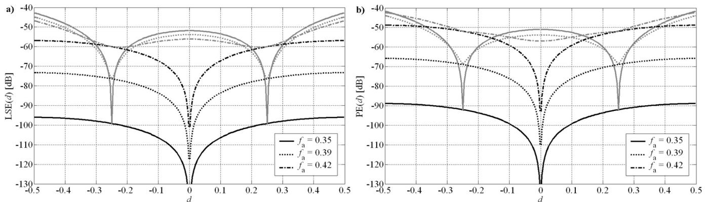
Fig. 10. Errors for VFD LS (a) and minimax (b) filters with  $N = 19$  (black lines) and their equivalents designed using asymmetric windows extracted for  $\epsilon_{ref} = 0.25$  without gain correction (gray lines).
