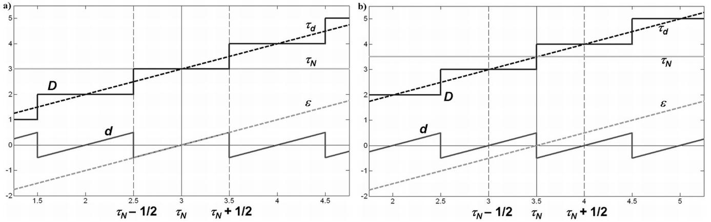
Fig. 2. Bulk delay  $\tau_N$ , net delay  $\epsilon$ , integer delay  $D$  and fractional delay  $d$  versus total delay  $\tau_d$  for fractional delay filters with lengths  $N = 7$  (a) and  $N = 8$  (b).
