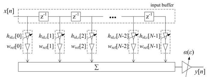
Fig. 1. The VFD filter implementation based on window method.  $x[n]$  and  $y[n]$  represent input and output signals, “ $z^{-1}$ ” blocks represent the unit delay elements storing input samples for one sampling period.
