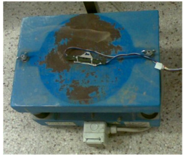
Fig. 15. Vibrating table with attached accelerometer.
